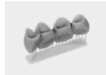
Support removal and finishing
