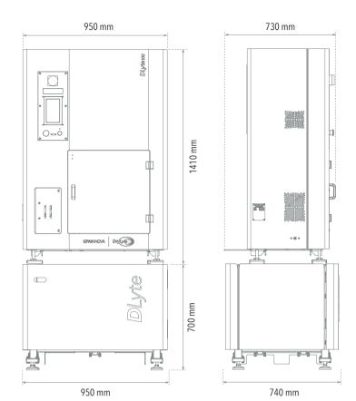
Consumption of 40 I/min. The air quality must be 1.5.1<sup>4</sup> according to ISO 8573 . (\*) Air quality required for a maintenance every 6 months (change of filters).
